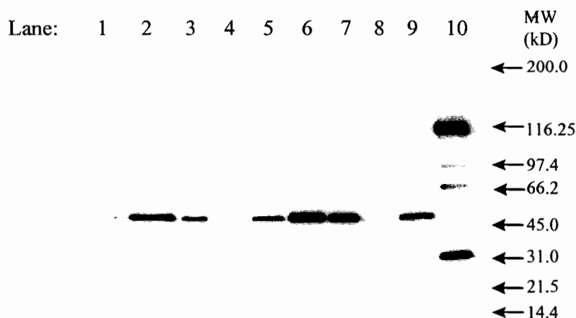
Figure 2. Western Blot Showing the Equivalence of CP4 EPSPS Protein Expressed by E. coli , Roundup Ready® Soybean and Roundup Ready® Corn Line NK603
