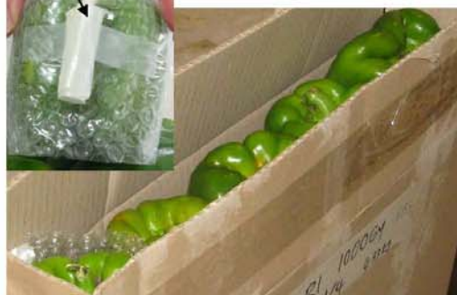
Figure 2. Capsicum and tomato arranged in a cardboard box ready for irradiation. Dosimeter attached to a piece of produce for monitoring doses received within the box.
