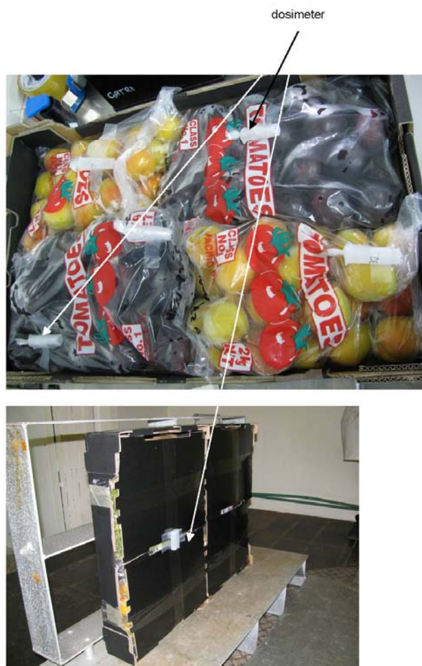
Figure 1. Plum and apricot fruits packed in plastic bags and placed in a cardboard carton ready for irradiation treatment. Dosimeter(s) attached to bags of fruit inside the carton and on outside of cartons.
