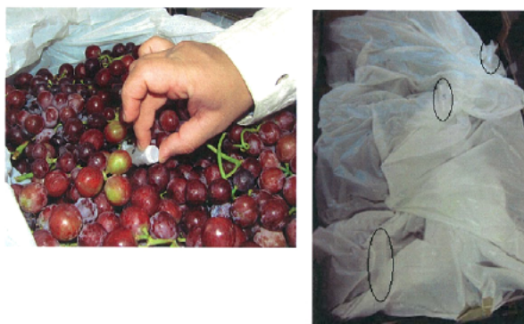
Figure 1: Trays of grapes for irradiation showing dosimeter position (circled).
