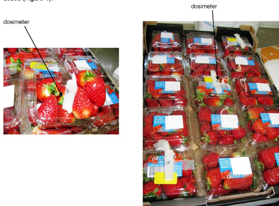
Figure 2. Punnets of strawberries in a cardboard box ready for irradiation. Dosimeter inside punnet and attached on the outside for monitoring doses received within the box. Source photos: ANSTO.
