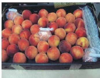
Figure 2: Tray of peaches for irradiation showing dosimeter position.
