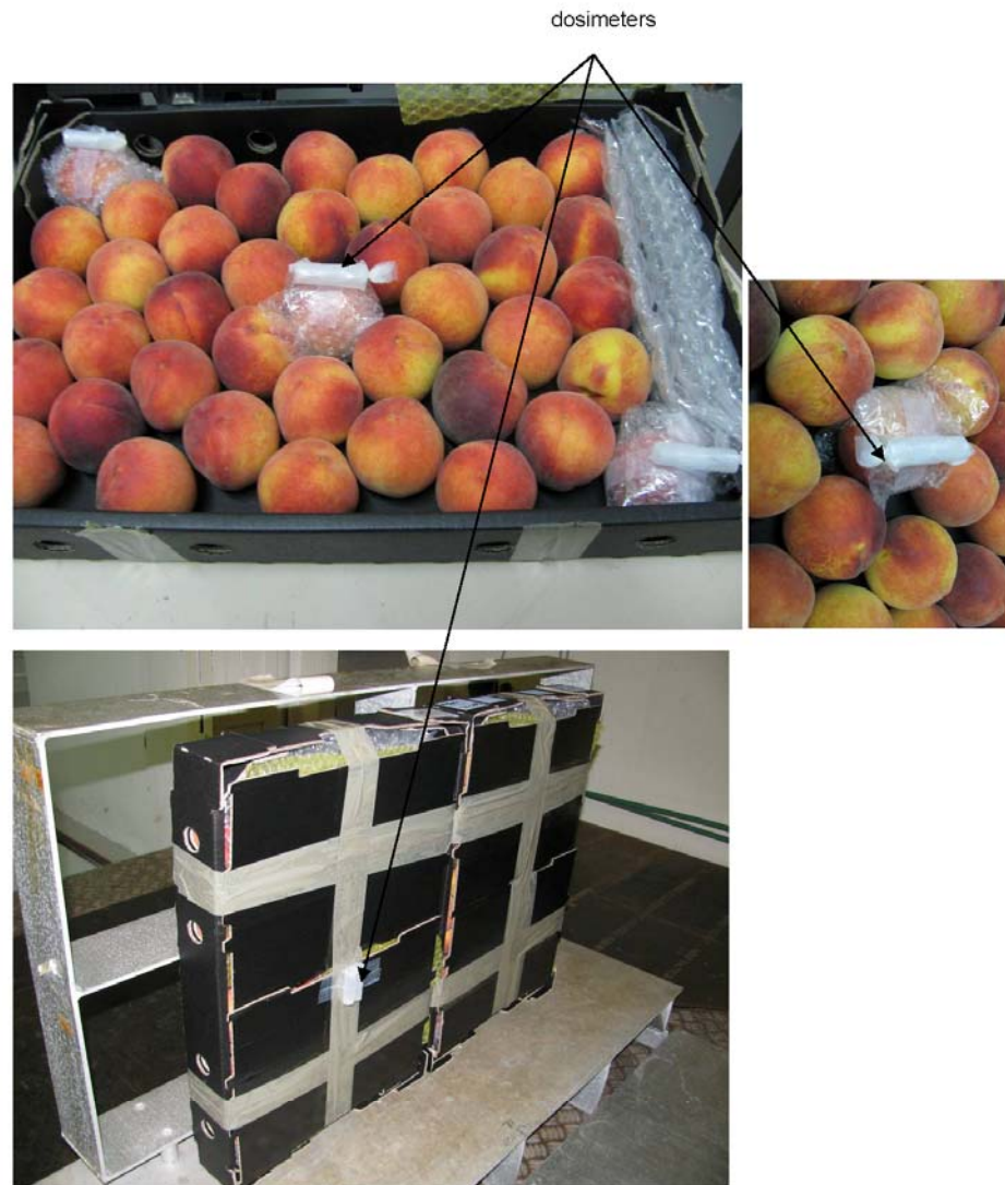
Figure 1. Peaches in a cardboard carton ready for irradiation treatment. Dosimeter(s) attached to fruit inside the carton and on outside of cartons. Source: Radiation Technology, ANSTO.
