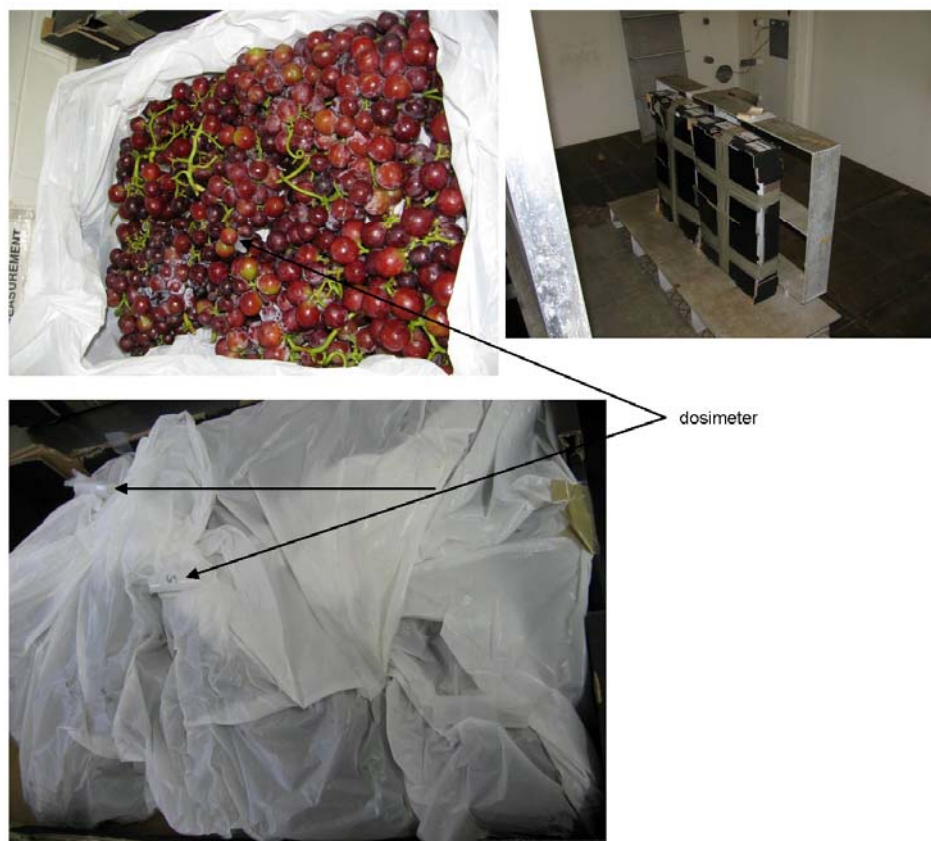
Figure 1. Table grapes packed in a plastic bag and placed in a cardboard carton ready for irradiation treatment. Dosimeter(s) were attached to bunches of berries inside the carton and on outside of the plastic bag for monitoring doses received within the box. Source: Radiation Technology, ANSTO.
