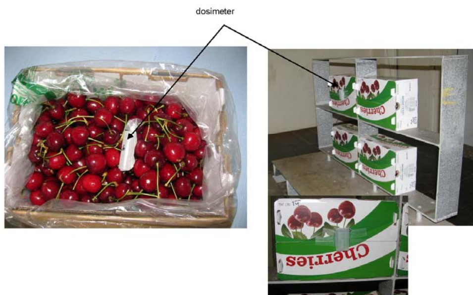
Figure 1. Cherry fruit packed in a lined 2 kg cardboard cherry carton ready for irradiation treatment. Dosimeter(s) situated inside the carton of fruit and on outside of cartons for monitoring doses received within the box. Source: Radiation Technology, ANSTO.
