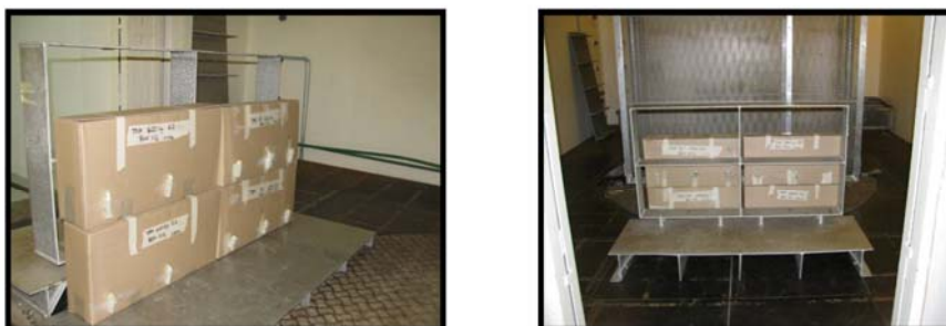
Figure 1. Boxes of produce positioned for irradiation. Dosimeters attached on the outside of boxes of packed produce.
