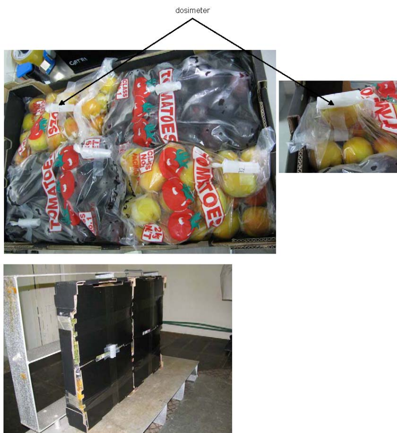
Figure 1. Apricot and plum fruits packed in plastic bags and placed in a cardboard carton ready for irradiation treatment. Dosimeter(s) attached to bags of fruit inside the carton and on outside of cartons for monitoring doses received within the box. Source: Radiation Technology, ANSTO.
