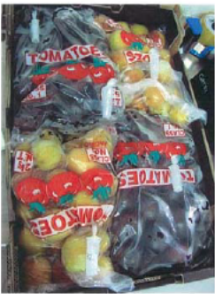
Figure 1: Dosimeters positioned on bags of apricots and plums.
