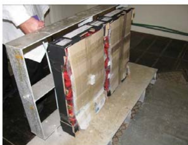
Figure 1. Boxes of strawberry positioned for irradiation. Dosimeters attached on the outside of boxes of packed punnets of strawberries. Source photo: ANSTO.
